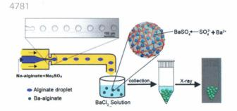
Microfluidic one-step fabrication of radiopaque alginate microgels with *in situ* synthesized barium sulfate nanoparticles
