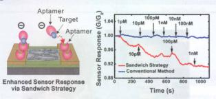
Aptamer sandwich-based carbon nanotube sensors for single-carbon-atomic-resolution detection of non-polar small molecular species
