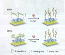
Analysis of DNA hybridization regarding the conformation of molecular layer with piezoelectric microcantilevers
