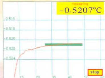
The freezing curve is shown on the graphic colour display during measuring.
