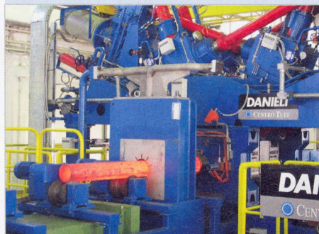
Prototype with three 4-roll stands at the Danieli R&D laboratories
