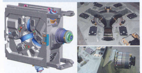
Stand-AUL: adjustable under load
