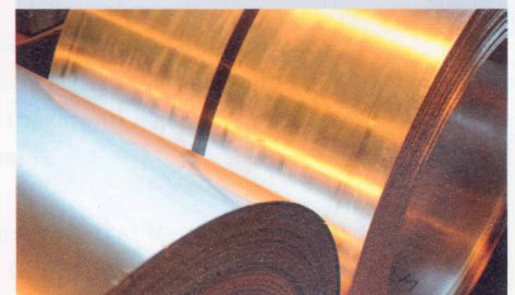
Hot rolled magnesium coils produced at MgF
