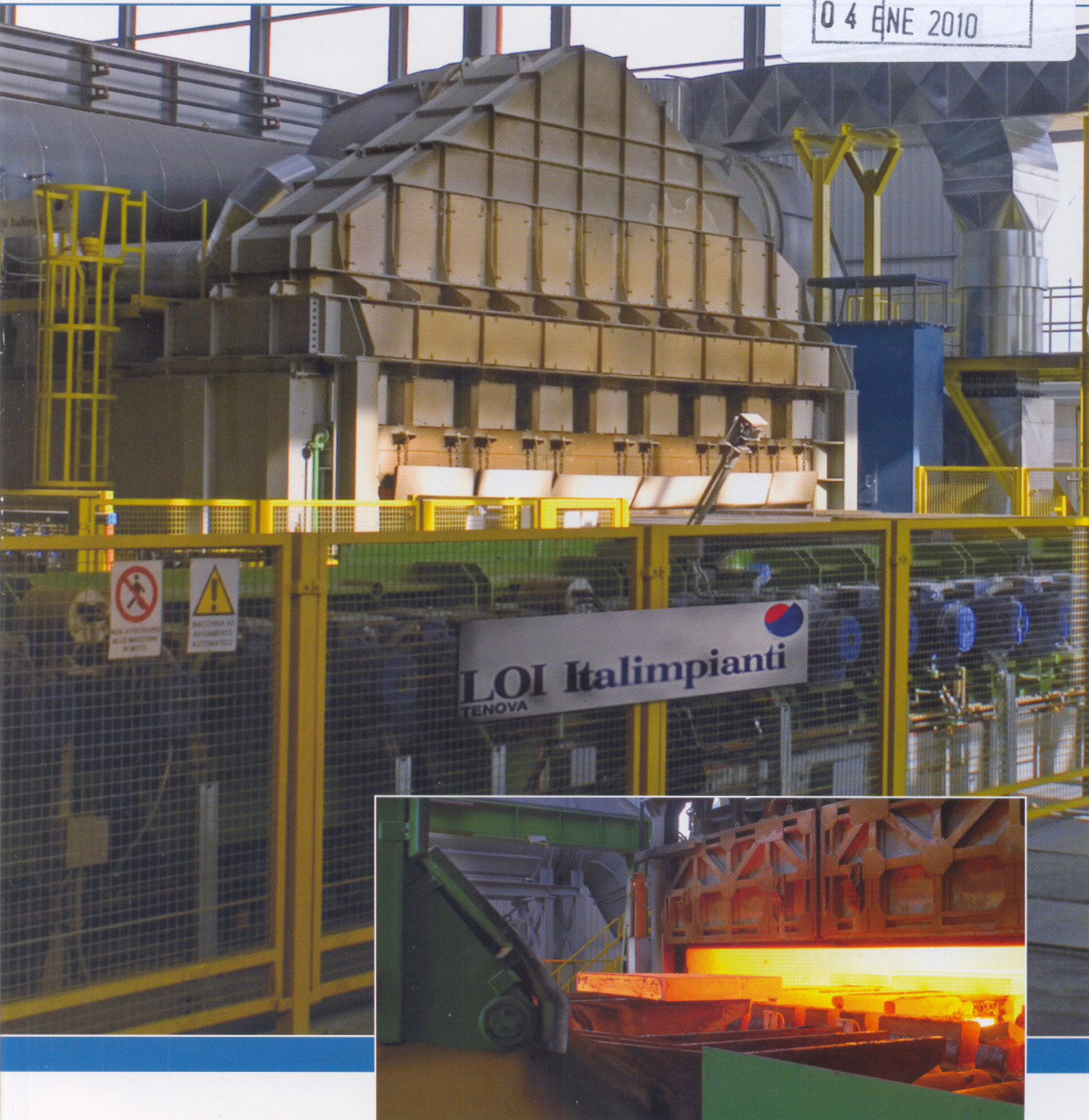
High-productivity pusher furnace at the Metinvest Trameal plate mill
