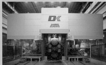
Combined 4-high/S6-high reversing mill
