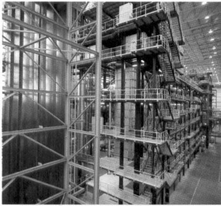
Cover photo: Looper and furnace section of the new hot dip galvanizing line at Voestalpine Stahl, Linz, Austria
