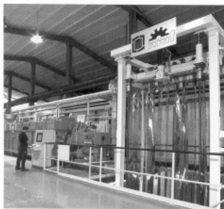
Cover photo: Strip accumulator and annealing zone of a bright annealing line
