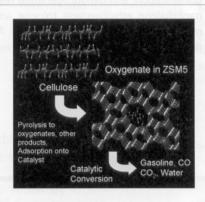
A fuelling success: High-quality aromatic fuel additives can be produced directly from solid biomass feedstocks by catalytic fast pyrolysis in a single catalytic reactor at short residence times. High heating rates and catalyst-to-feed ratios are needed to ensure that pyrolized biomass compounds enter the pores of the ZSM5 catalyst and that thermal decomposition is avoided. Product selectivity is a function of the active site and pore structure of the catalyst.
