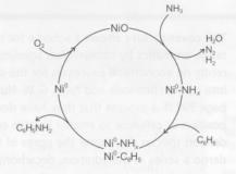
Suspended amination: Semi-batch oxidative synthesis of aniline from benzene and ammonia was performed at atmospheric pressure using a NiO/ZrO<sub>2</sub> cataloreactant in a microreactor flow setup. A Langmuir–Hinshelwood mechanism is suggested based on the surface reaction between adsorbed benzene- and ammonia-derived NH<sub>x</sub> species on metallic Ni surface sites.
