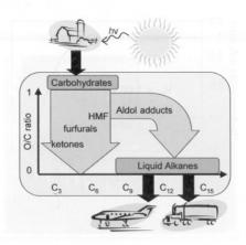
Right on target: Transportation fuels can be directly produced from renewable biomass resources by converting carbohydrates into alkanes with targeted molecular weights, such as C<sub>8</sub>–C<sub>15</sub> for jet-fuel applications. Targeted alkanes can be produced from a variety of biomass-derived carbonyl compounds, such as fructose, 5-hydroxymethylfurfural, 5-methylfurfural, 2-furaldehyde, and acetone.
