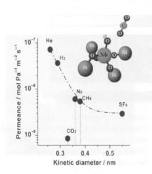
Stayin' in the membrane: A microporous composite membrane composed of niobia and silica shows an exceptionally low permeability for carbon dioxide despite its small size. Other small molecules such as hydrogen, methane, oxygen, and nitrogen can pass much more easily. Nb-bound hydroxy groups probably act as strong adsorption sites for carbon dioxide. Such a gas-selective ceramic membrane may be useful to separate CO<sub>2</sub> from gas mixtures.
