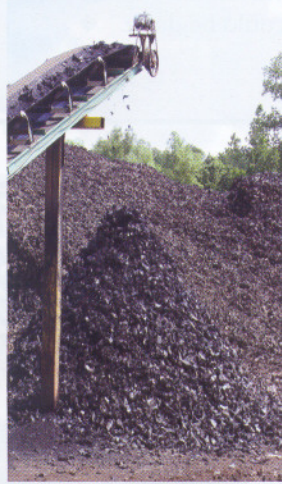
Material off the belt of the Saturn 62-40HT is used for TDF or as a crumb rubber feedstock
